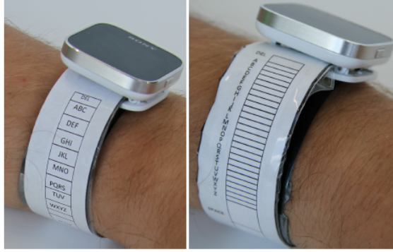
Figure 2.16: Using a touch-sensitive wristband for text entry on smartwatches [17]. The multi-tap layout is shown on the left and the linear keyboard is shown on the right.
