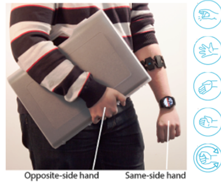
Figure 2.24: Control smartwatch using Myo armband [25].
