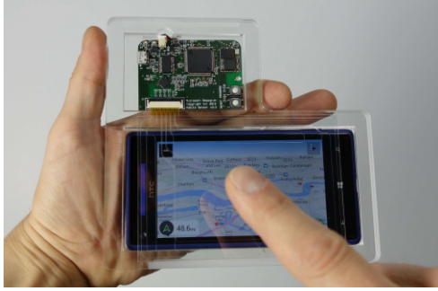
Figure 2.7: Electric field sensing based interactions with mobile devices [8].
