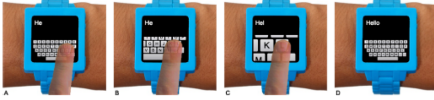
Figure 2.9: (a) Default ZoomBoard layout [10]. (b & c) User taps for iterative zooming. (d) The keyboard resets after entering the desired character.
