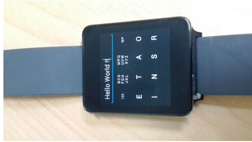
Figure 5.2: ETAO Keyboard prototype running on LG W100 smartwatch.
