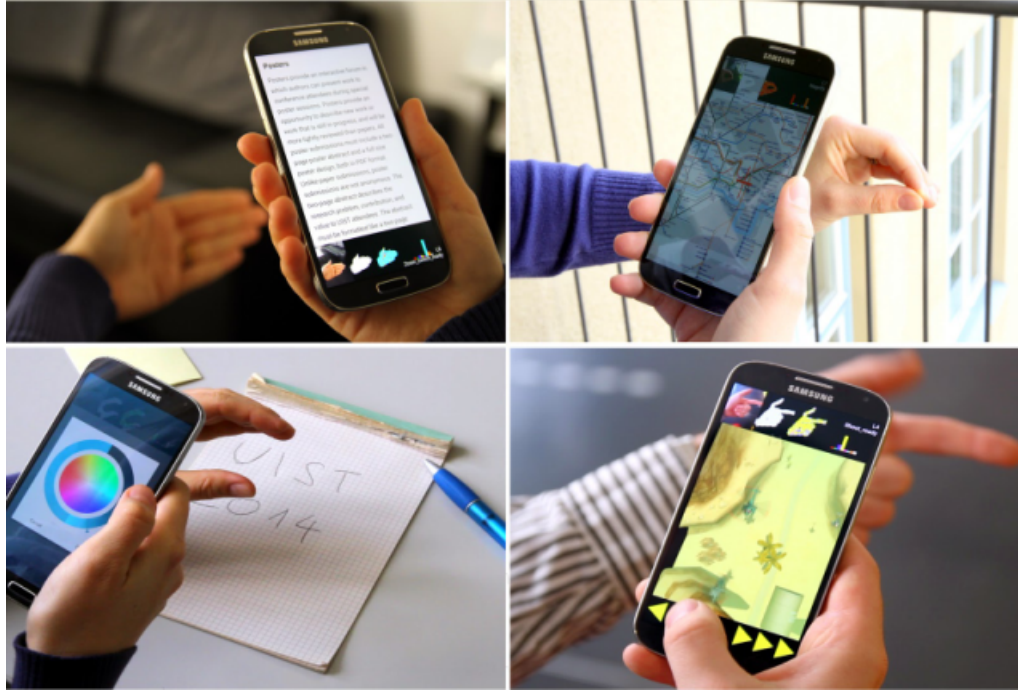
Figure 2.4: Recognizing different in-air hand gestures using Phone’s RGB camera [5].
