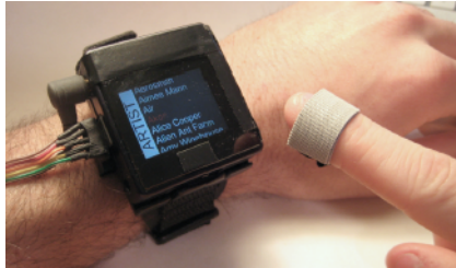
Figure 2.20: Around device interaction with smartwatches using magnetometer sensor [21].
