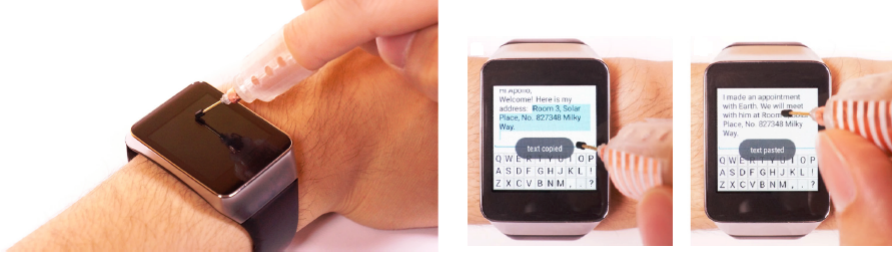
Figure 2.17: Interaction with smartwatch using ‘NanoStylus’ prototype [18].
