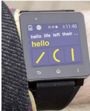
Figure 2.14: UniWatch Keyboard: Typing using three strokes ('/', '(', '|') [15].
