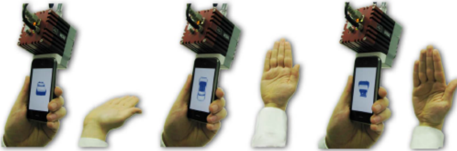
Figure 2.6: PalmSpace prototype detects different palm poses using depth camera [7].
